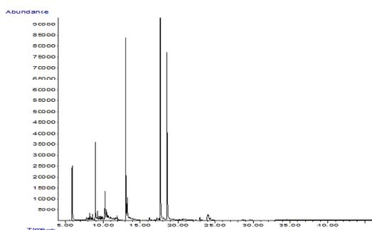
**Fig .2. Example mass chromatogram of the BS NQ30MPAH SIM M method on sample number L8 from Leeds**
